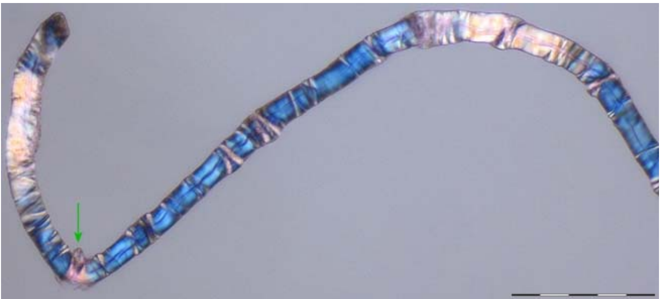
Fig 19 Linen fiber showing distinct dislocations and a fracture with buckling (green arrow), see fig 20; p, scale bar 50 \mu m
