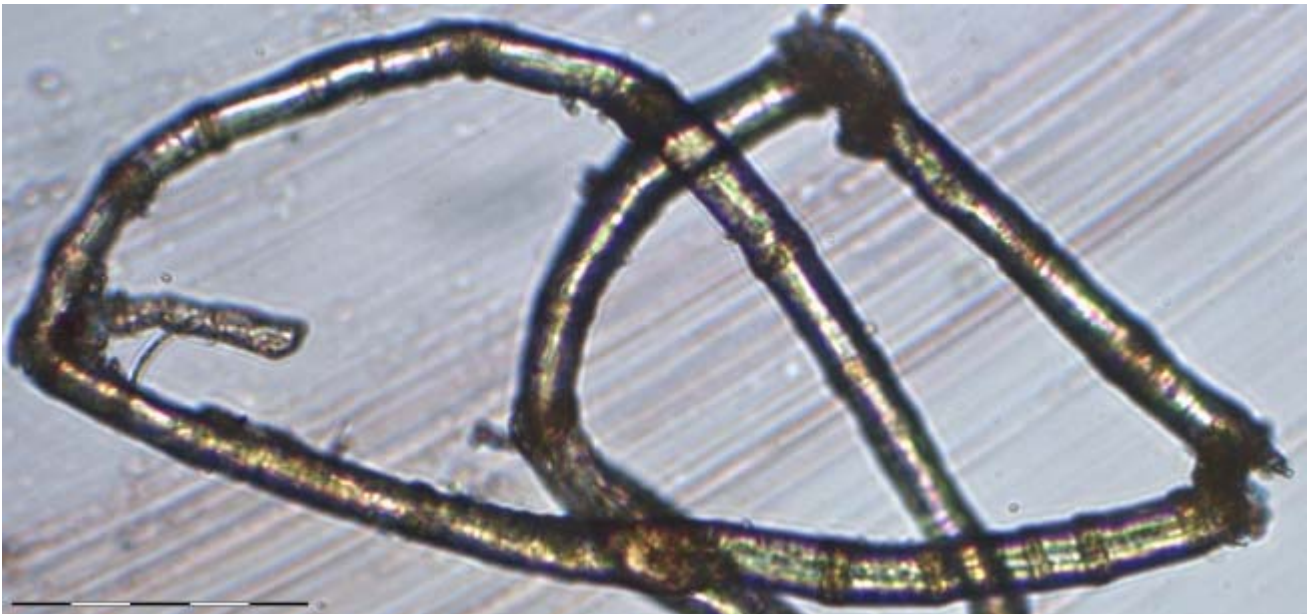
Fig 23 Linen fiber with loops formed by bending in segments at dislocation level. The pink striated background is an artefact from a pencil; bf, scale bar 50 \mu m
