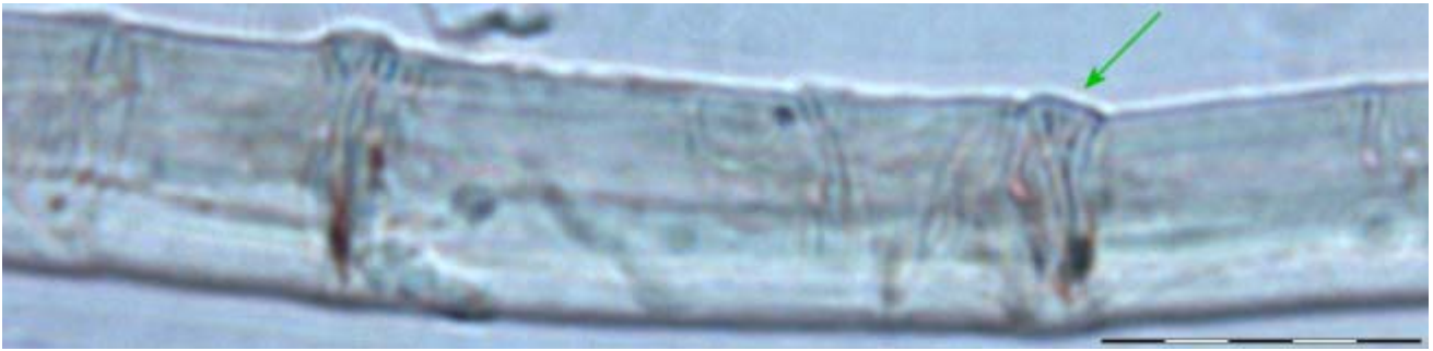
Fig 18 Arrow pointing at buckling; pc, scale bar 20 \mu m
