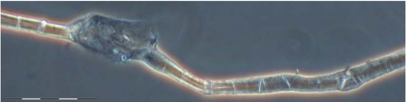
Fig 26 A rectangular thickening of the fiber most probably formed by squeezing, cf. fig 27; pc, scale bar 50µm
