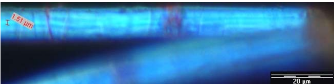
Fig 9 Left “leg” with bundles of fibrils; their individual thickness indicated by red writing. The image of the fiber has been rotated 28 degrees clockwise compared to fig 8; p
