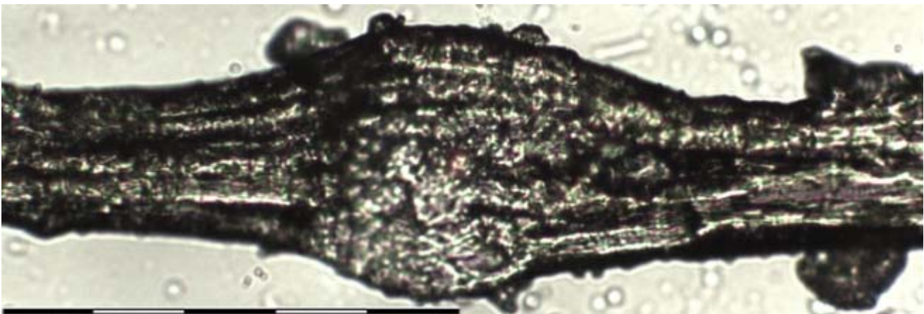
Fig 27 Squeezing of a dry hemp fiber by tweezers. Note the thickening; bf, scale bar 100µm. Courtesy of L.G. Thygesen
