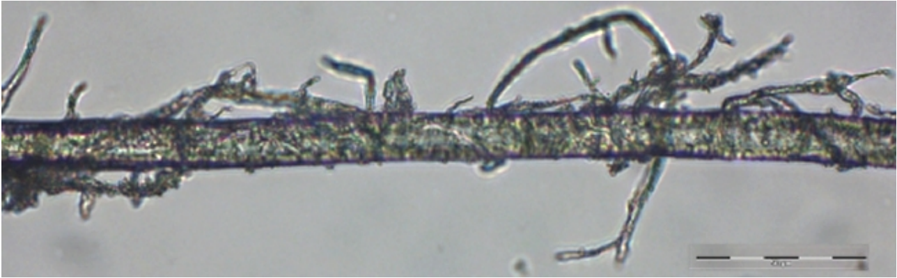
Fig 1. Frayed part of fiber; bf, scale bar 50µm
