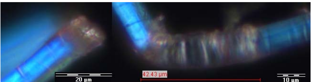
Fig 10 The image to the left represents the “open” fracture. The image to the right represents the bending area surrounded by cell debris; p
