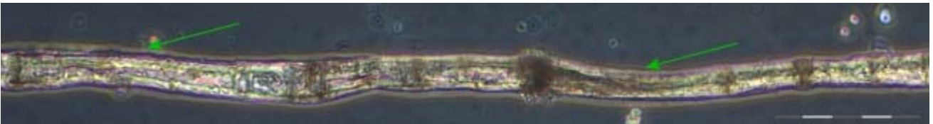
Fig 30 Narrowing of fiber; pc, scale bar 50 \mu m
