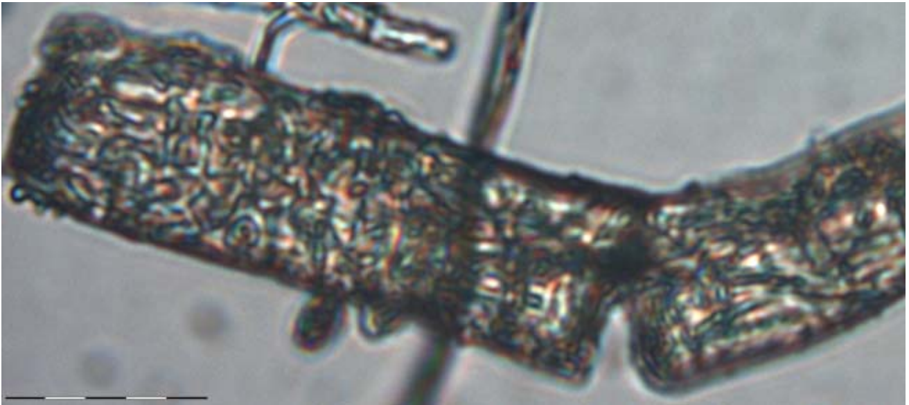
Fig 41 Surface layer of a flax fiber. Note the snake-like structure and compare it to fig 45, bf; scale bar 20 \mu m
